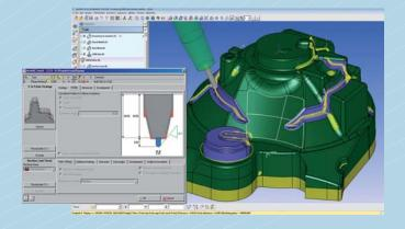
Re-engineered 'Auto 5' module: WorkNC's Auto 5 automatically converts 3-axis toolpaths into simultaneous 5-axis toolpaths. The Auto 5 module has been re-engineered with the introduction of an even more powerful calculation engine associated with a new collision detection and avoidance module. The improved calculation times can be 3 to 5 times
